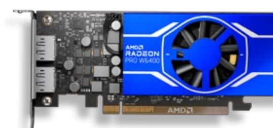
Option 01: Short bracket for Small Form Factor (SFF) systems.
