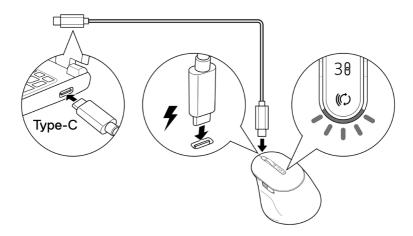
The white low battery LED indicator will breathe until the battery is fully charged or the USB charging cable is unplugged.
